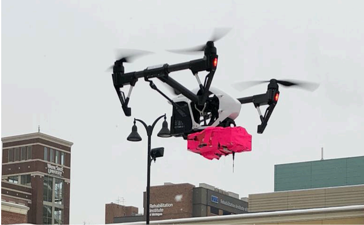
Figure 43: The UAS flying during the experiment with the radio transceiver and the GPS receiver inside the pink box. The radio antenna pointed down.
