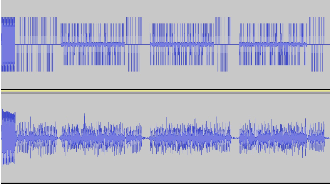
Figure 14: The MSD signal sent by the IVS and the received MSD signal at the input of the laboratory PSAP center.
